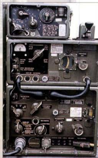
Fig. 2: The RA-200 back-pack set. The antenna tuning unit is at the top, with transmitter immediately below, and the receiver at the bottom.
