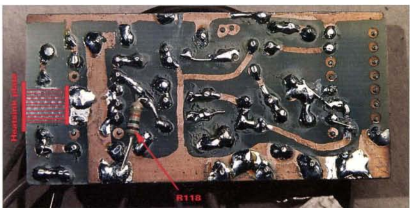
Fig. 3: Audio output and tone burst board viewed from the prototype track side. The combined fixing tag and heatsink is normally attached, but is removed for photographic purposes (see text).
